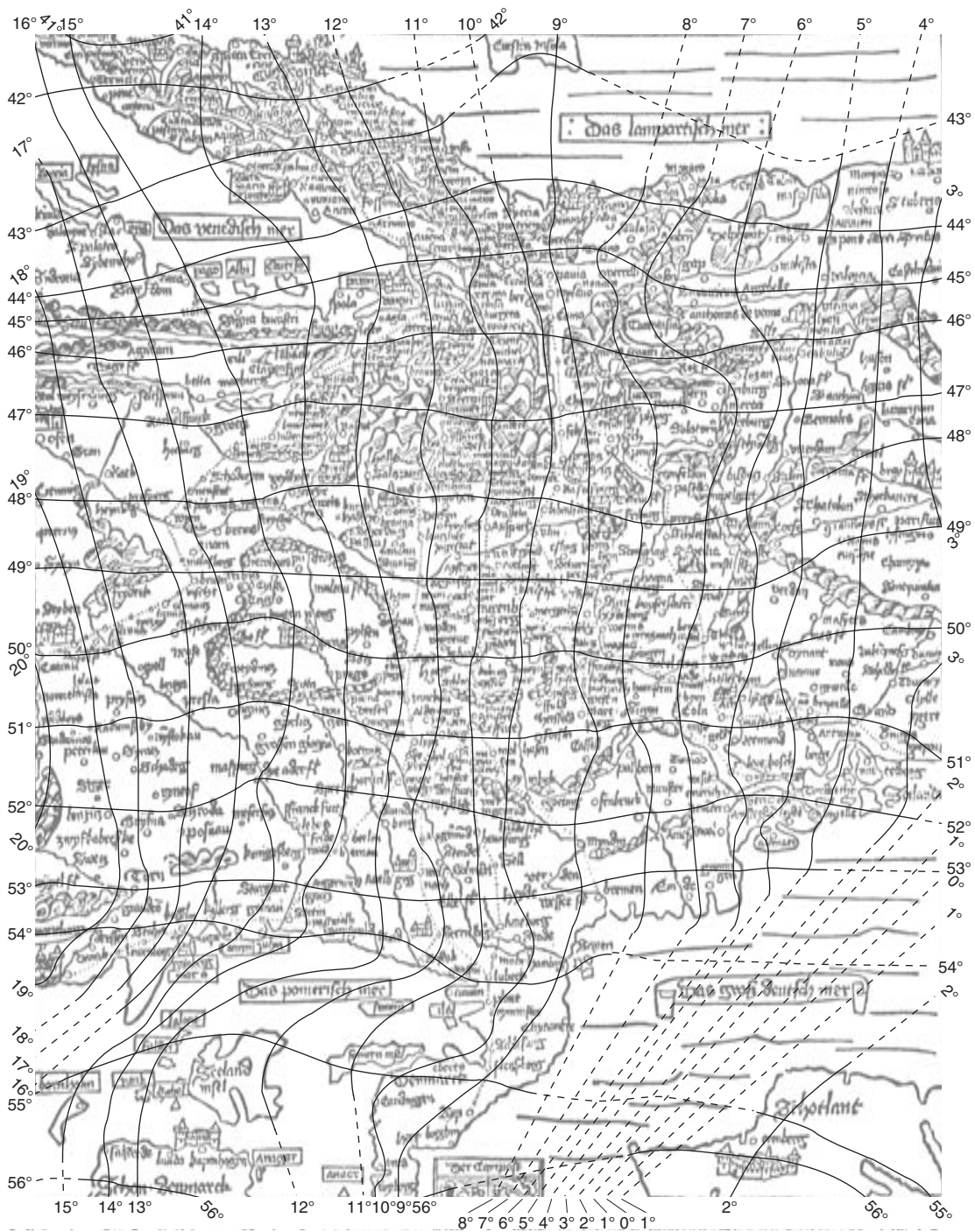
FIG. 42.12. DISTORTION GRID, ETZLAUB'S ROM WEG MAP. South is at the top (see pl. 44). The varying accuracy reveals some of Etzlaub's compilation work. The depiction of the central area was based on fairly good primary data (distances and latitudes), whereas the outer areas were mainly copied from maps in the 1482 Ulm edition of Ptolemy's Geography .
