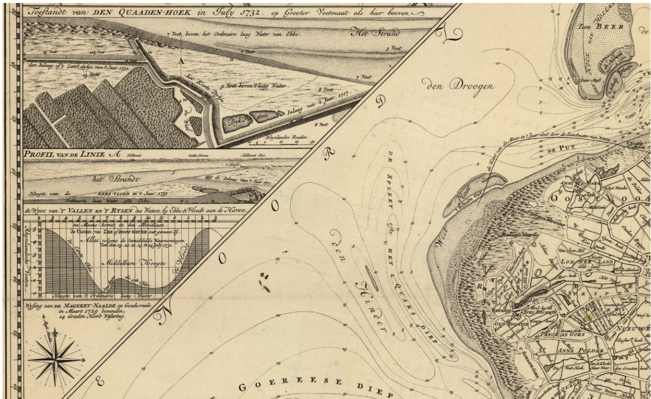
FIG. 190. DETAIL FROM NICOLAAS SAMUELSZ. CRUQUIUS, HET EYLANDT WEST-VOORN OF GOEREDEE MET DE DIEPTENS EN DE DROOGTENS RONS-OMME (1733), 1:54,000. Detail from Cruquius's map of the island of Goeree and surrounding waters showing the insets depicting the endangered coast (with normal high tides and the inundations of 1717 and 1732), the pattern of
