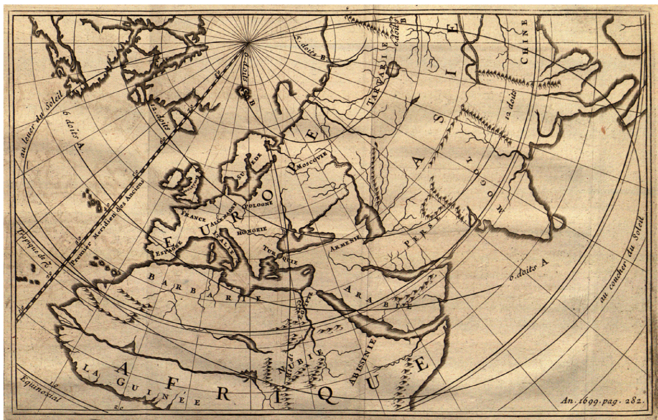
FIG. 210. CASSINI I'S UNTITLED MAP OF THE SOLAR ECLIPSE OF 23 SEPTEMBER 1699. From sunrise to sunset, Cassini mapped lines of centrality (twelve digits), partial eclipse (six digits), and the limits of the eclipse. The projection is a normal aspect azimuthal equidistant. From Jean-Dominique Cassini, “Reflexions sur l’eclipse du 23. Septembre
