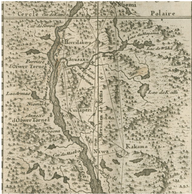
FIG. 273. DETAIL FROM THE CARTE DE L'ARC DU MERIDIEN MESURE AU CERCLE POLAIRE, 1738. From Pierre Louis Moreau de Maupertuis, La figure de la Terre, déterminée par les observations (Paris: Imprimerie Royale, 1738), following p. 184. Detail showing the line of the meridian (“Meridien de Kittis”), the horizontal double line of the Arctic Circle (“Cercle Polaire”), the baseline measured across the frozen river (“Base de 7406 [toises] 5 [pieds] 2 [pouces]”), and the central portion of the geodetic triangulation. See figure 436 for a map of the entire triangulation. Size of the entire original: ca. 17 × 10 cm; size of detail: ca. 8.4 × 8.4 cm. Image courtesy of the Special Collections Library, University of Michigan, Ann Arbor (QB 283 .M45).
