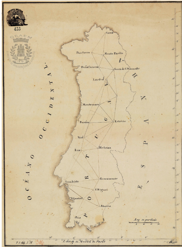
FIG. 271. FRANCISCO ANTÓNIO CIERA, MAP OF THE POINTS AND THE SERIES OF TRIANGLES FOR MEASURING THE DEGREE OF THE MERIDIAN BETWEEN 37^{\circ} AND 43^{\circ}45'N , 1791. Manuscript, ca. 1:2,000,000. The first geodetic network of Portugal, designed and signed by Ciera, based on the surveys of 1790–91 directed by him. Size of original: 49 \times 40 cm. Image courtesy of Portugal/Gabinete de Estudos Arqueológicos da Engenharia Militar/Direção de Infraestruturas do Exército, Lisbon (4361/I-4-49-82).
