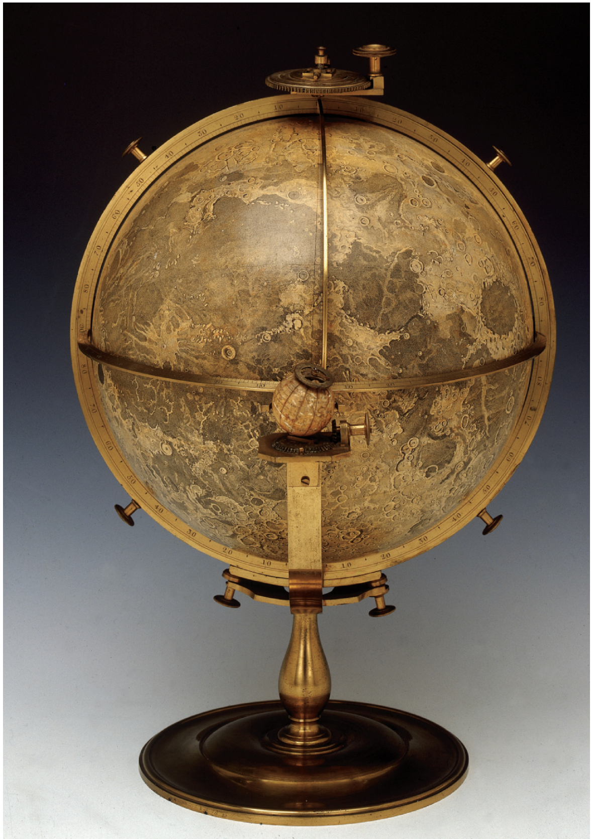
FIG. 335. JOHN RUSSELL'S SELENOGRAPHIA , 1797. The gores of this lunar globe were printed from stipple-engraved plates and hand-colored. Not shown in this image is the unseen far side of the moon, which Russell of course left blank. Russell placed a small terrestrial globe on a separate gear in
