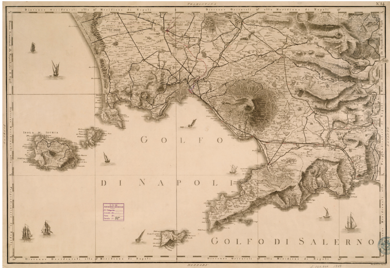
FIG. 270. GIOVANNI ANTONIO RIZZI ZANNONI, GULF OF NAPLES, 1794. From his Atlante geografico del Regno di Napoli (Naples, 1788–1812), foglio 14, scale ca. 1:114,000. From 1781 onward Rizzi Zannoni was the first to undertake systematic geodetic surveys in southern Italy.
