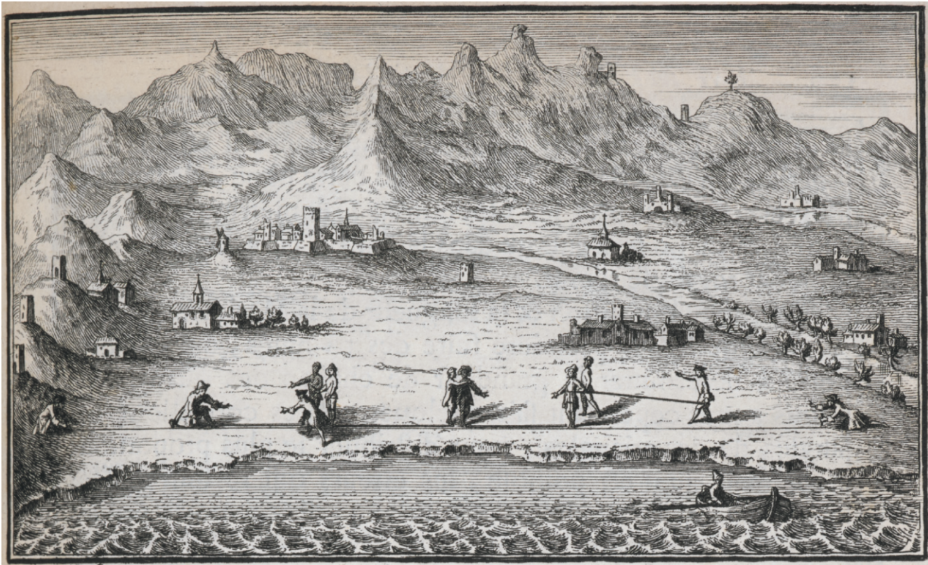
FIG. 260. MEASURING A BASELINE WITH WOODEN RODS. This illustrative vignette shows the early method of measuring a baseline by laying wooden rods on the ground, one set against another, along a stretched-out rope; each rod
