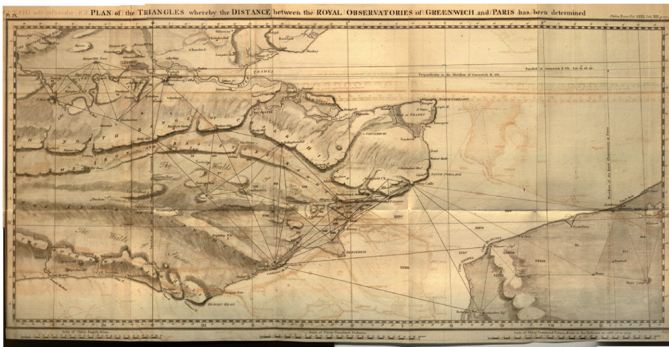
FIG. 344. PLAN OF THE TRIANGLES WHEREBY THE DISTANCE BETWEEN THE ROYAL OBSERVATORIES OF GREENWICH AND PARIS HAS BEEN DETERMINED. From William Roy, "An Account of the Trigonometrical Operation, Whereby the Distance between the Meridians of the Royal Observatories of Greenwich and Paris Has Been
