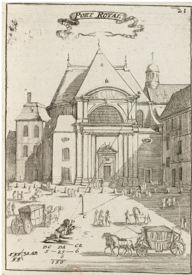
FIG. 364. THE USE OF SIMILAR TRIANGLES TO FIND A SINGLE UNKNOWN LENGTH. To find the height of the wall, AB, the surveyor places a vertical stick CE in the ground and then finds point D such that E and B are aligned; the triangles ECD and BAD are similar, so the ratios of their sides will be the same: DC/CE = DA/AB . The lengths DC and DA are measured, CE is known, so AB can be calculated as DA \times CE/DC , as shown in the lower left corner. From Manesson-Mallet 1702, 21 (pl. 9).
