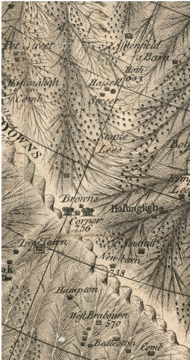
FIG. 350. SOME OF THE SPOT HEIGHTS ON CHRISTOPHER PACKE'S A NEW PHILOSOPHICO-CHOROGRAPHICAL CHART OF EAST-KENT (LONDON, 1743). Packe determined all his heights in feet above sea level with a portable barometer compared against a stationary barometer of similar manufacture kept at his home; he calibrated his portable barometer against the height of the main tower at Canterbury Cathedral. Note that Packe disturbed the planimetric form of his map with only a few lines of imprecise hills drawn in profile to indicate the main ridge lines. Otherwise he delineated the courses of streams and rivers so he could readily locate spot heights precisely. The full four-sheet map is reproduced as figure 622. Size of each sheet: 60 × 65 cm; size of detail: ca. 16.0 × 8.5 cm. Image courtesy of the National Library of Scotland, Edinburgh (EME.s.130).
