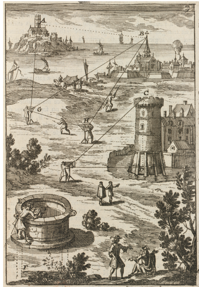
FIG. 365. THE KINDS OF TRIANGLES THAT COULD BE SOLVED WITH TRIGONOMETRY. In the middle of this image, an unmarked observer (who for convenience can be labeled as J) is shown forming a single triangle with a vertical tower. If the distance JD from the observer to the tower is known, then the height of the tower CD is JD \times \text{tangent}(\text{vertical angle at J}) . At the rear of the image, the measured horizontal angles at G and H and baseline GH can be used to determine the lengths of the sloping sides GB and HB via the law of sines: HB = GH \times \text{sine}(\text{angle at G}) \div \text{sine}(\text{angle at B [i.e., } 180^\circ - G - H]) . From these sides, plus the vertical angles from G or H to B, the surveyor can then calculate the horizontal distance, from G, as GB \times \text{sine}(\text{vertical angle at G}) , and the vertical distance, from G, as GB \times \text{cosine}(\text{vertical angle at G}) . Those results can then be used in a similar manner to determine horizontal and vertical distances from both B and G to A. From Manesson-Mallet 1702, 3 (pl. 1).
