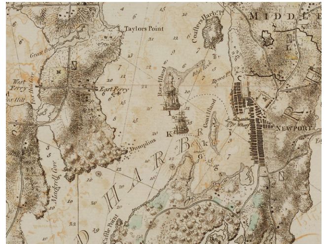
FIG. 502. DETAIL FROM A CHART OF THE HARBOUR OF RHODE ISLAND AND NARRAGANSET BAY [LONDON] CA. 1780; FIRST PUBLISHED 1776. Scale, ca. 1:51,400 (41°40'N). Originally surveyed by Charles Blaskowitz, Thomas Wheeler, and others, working for Samuel Holland, this is one of the charts in J. F. W. Des Barres's monumental four-volume Atlantic Neptune (1780) and shows an impressive density of soundings, not only in the bays and estuaries but also along the banks. Yet the station points in the sea are not positioned according to trigonometric determinations on land, as might be expected from Holland, who was a military geographical engineer and whose marine cartography focused particularly on the coastline visible from the sea. The ships are those of the French and British forces at the moment of Admiral Charles-Henri d'Estaing's arrival in the estuary 29 July 1778. Size of the entire original: 106.5 × 74.5 cm; size of detail: ca. 12.5 × 16.5 cm. Image courtesy of the Bibliothèque nationale de France, Paris (Cartes et plans, Ge BB 203, vol. 3, no. 14).
