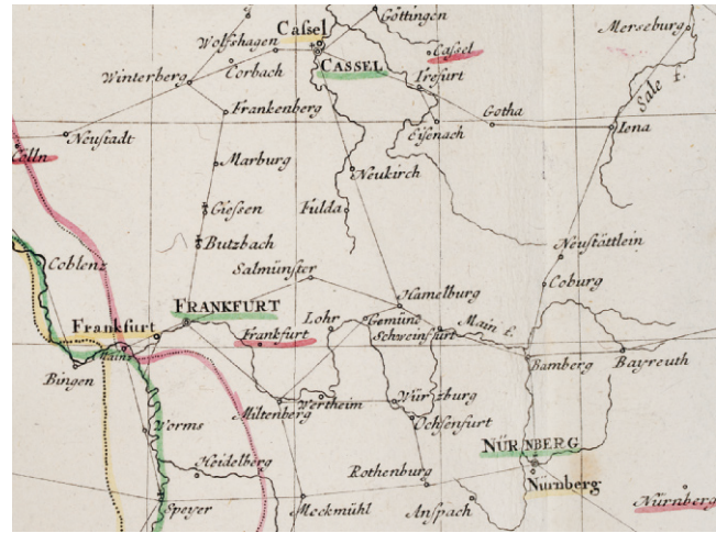
FIG. 532. DETAIL FROM TOBIAS MAYER’S GERMANIAE ATQVE IN EA LOCORVM PRINCIPALIORVM MAPPA CRITICA (NUREMBERG: HOMANN HEIRS, 1750). Mayer contrasted the locations of key places (e.g., Cassel, Nuremberg, Frankfurt) and boundaries according to existing maps of Germany by the Homann Heirs (red) and Guillaume Delisle (yellow) with recently determined latitudes and longitudes (green).
