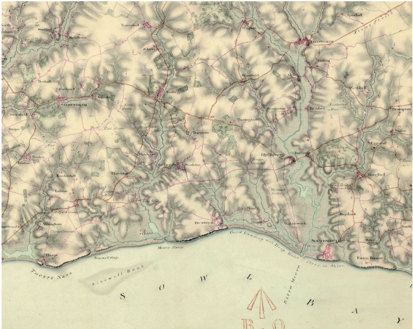
FIG. 565. DETAIL FROM A MAP OF THE COAST OF EAST ANGLIA BETWEEN WINTERTON NESS AND FELIXSTOWE, TOGETHER WITH A DEEP HINTERLAND, ENDORSED BY GEORGE PINK, CHIEF MILITARY SURVEYOR, 1798. Although based on existing published commercial mapping by William Faden and Joseph Hodkinson, the landscape is shown in a style that represents the terrain from a military point of view in such a way that the eye can instantly grasp the minutiae of hills, marshes, and coastal dunes and cliffs. Roads are classified according to their passability
