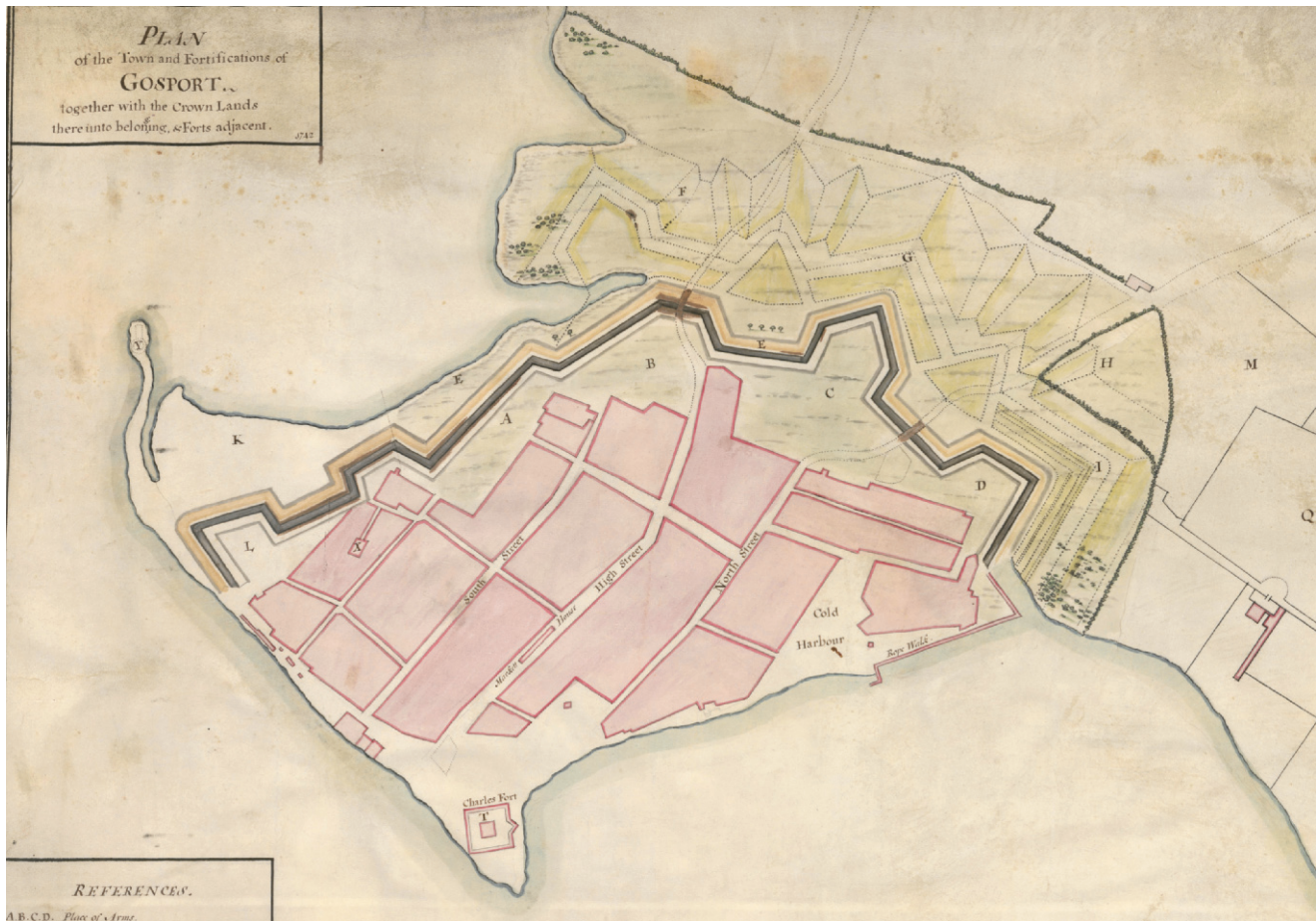
FIG. 564. BOARD OF ORDNANCE HOUSE STYLE OF DRAFTSMANSHIP BY BRITISH ENGINEERS. The Board of Ordnance developed a distinctive house style, as in this detail from the anonymous “Plan of the Town and Fortifications of Gosport, Together with the Crown Lands thereunto Belonging, and Forts Adjacent” (1742); proposed new outworks are
