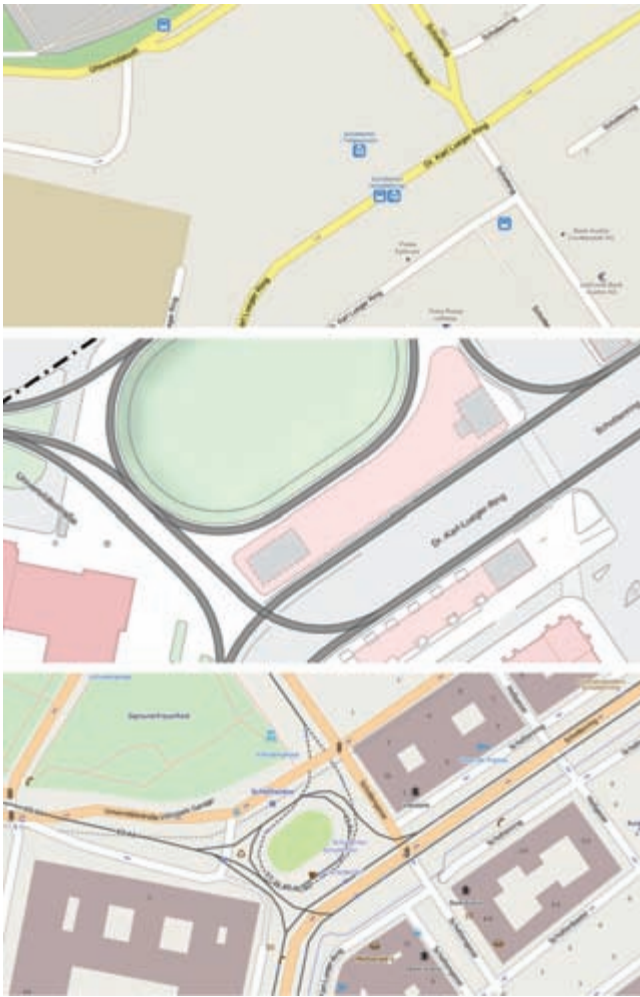
FIG. 1123. WAYFINDING-RELEVANT DIFFERENCES IN DATA QUALITY. Shown are the maximum zoom levels of three services: commercial service Google Maps (top), public service ViennaGIS (middle), and OpenStreetMap (bottom). Images courtesy of Google Maps (top) and ViennaGIS (middle). © OpenStreetMap contributors (bottom).
