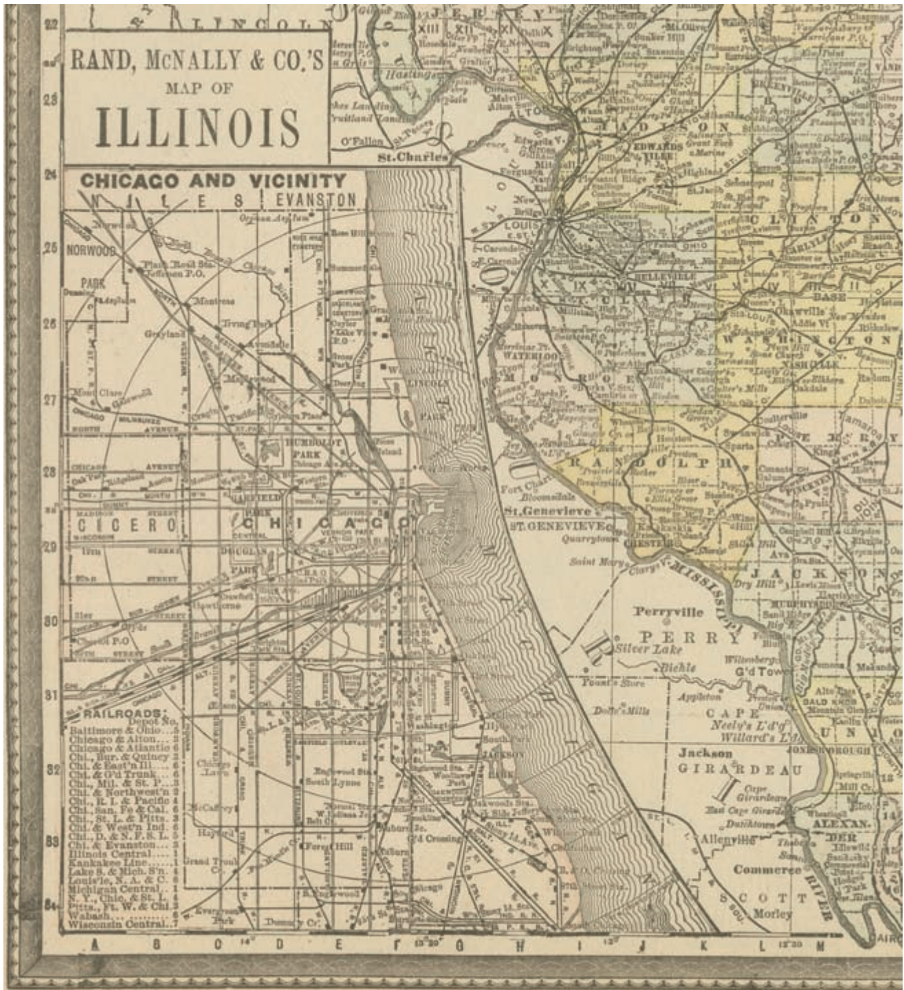
FIG. 1095. "CHICAGO AND VICINITY" MAP INSET ON RAND, McNALLY & CO.'S MAP OF ILLINOIS. This detail of Chicago from an Illinois map in an 1890 Rand McNally atlas illustrates the small size and precise placement of stamped type lettering in wax engraving.
