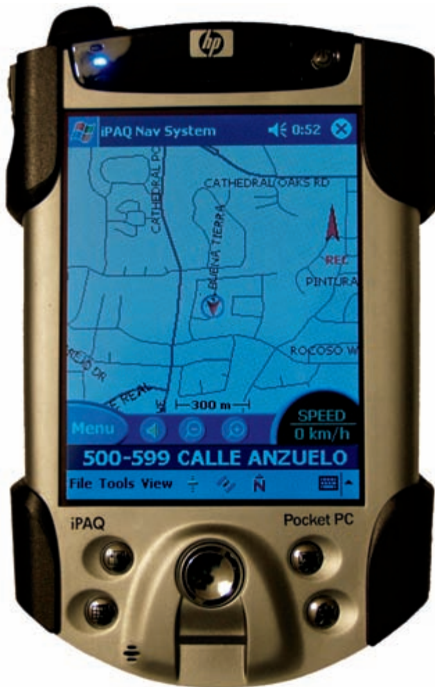
FIG. 1109. HEWLETT PACKARD NAVIGATION SYSTEM FOR THE iPAQ PERSONAL DIGITAL ASSISTANT. The screen is 240 \times 320 pixels. Many street names are suppressed, but the system accurately reports the vehicle parked on the 500 block of Calle Anzuelo. Image courtesy of Val Noronha.
