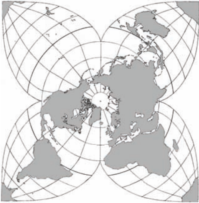
FIG. 1134. WILLIAM WILLIAM-OLSSON'S POLAR PROJECTION FOR WORLD MAPS PUBLISHED IN 1968. The central part is based on the Lambert equal-area azimuthal projection and extended to the parallel circle 20°N. To that four Bonne lobes adapted from the Werner projection are added. The lobes are extended east-west to fit the central projection and north-south to give the projection an equal-area capacity. In the figure, the central meridian is placed for an optimal view of Europe with the central point at London.
