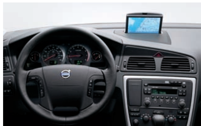
FIG. 1111. IN-VEHICLE DASHBOARD DISPLAY. Many built-in navigation displays are positioned in the center console, near the radio. In this vehicle, a 2005 Volvo V70, the navigation panel is on the top of the dashboard, minimizing eye diversion.
