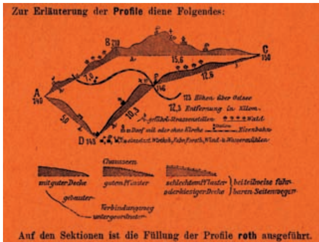
FIG. 1098. INSTRUCTIONS FOR THE PROFILES IN ROBERT MITTELBACH'S DEUTSCHE STRASSENPROFILKARTE FÜR RADFAHRER , CA. 1890–1900. Detail from loose leaf inside slipcase of folded map showing sample elevation profiles with differently shaded road quality classes, distances between points indicated, and elevations given for points A–D. The instructions also include comprehensive explanatory text (which has been omitted in this detail). Size of the entire original: 31.5 × 13 cm; size of detail: ca. 6.9 × 9.2 cm. Image courtesy of Wolfgang Lierz.
